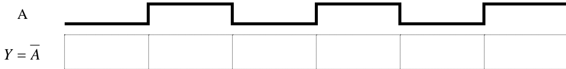
Figure 4.1 – Time diagram for a NOT gate
